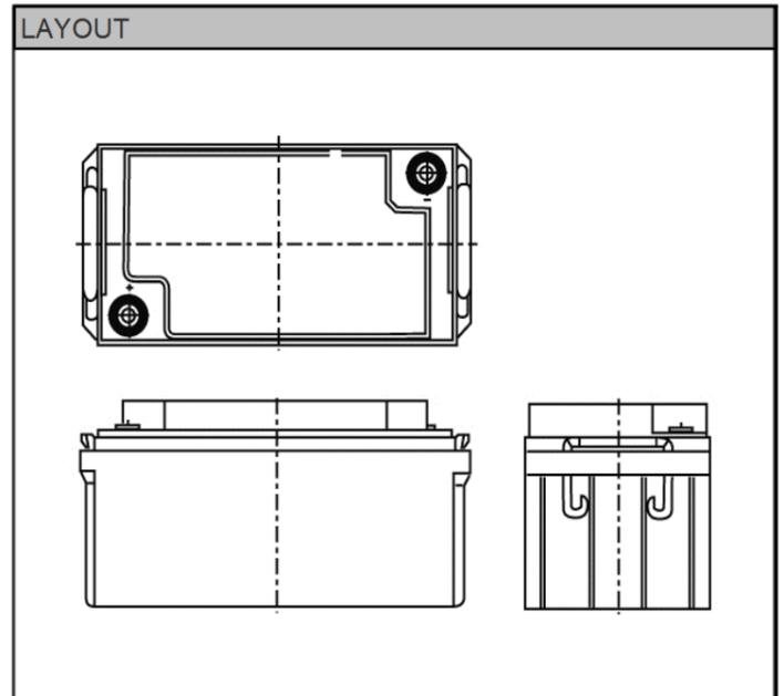
This battery type must never be installed suspended by their handles
